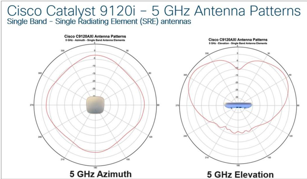
9120i secondary 5-GHz single-band antenna patterns
