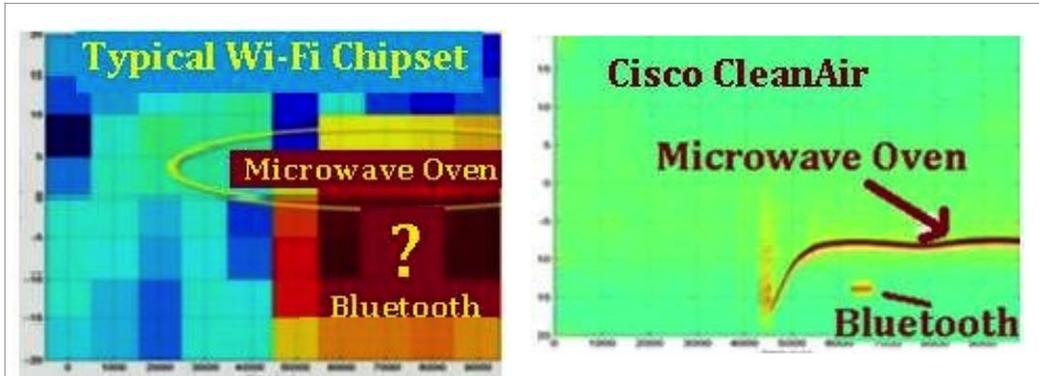
CleanAir clearly identifies the interference using dedicated radio and custom silicon
