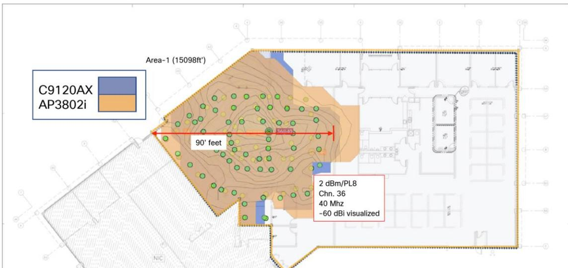
Comparison of C9120 and AP3802i coverage patterns as measured over the air
