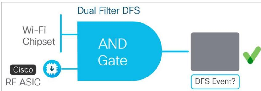
DFS event (detected by Wi-Fi chipset) is compared to RF ASIC to verify it is indeed a real DFS event
