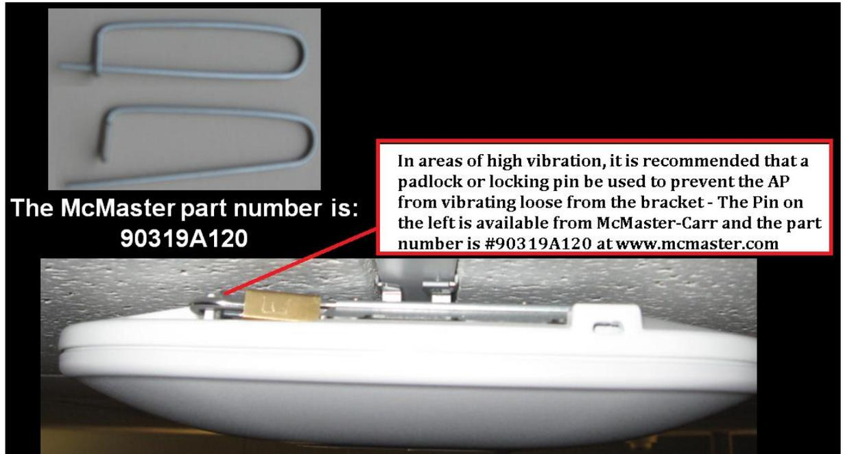
A metal pin or padlock will not deteriorate over time so it is better than a plastic tie
