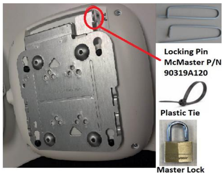
Figure 6. Securing the AP
