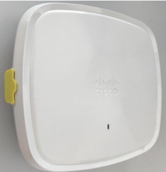
Figure 26. 9130E showing antenna connector
