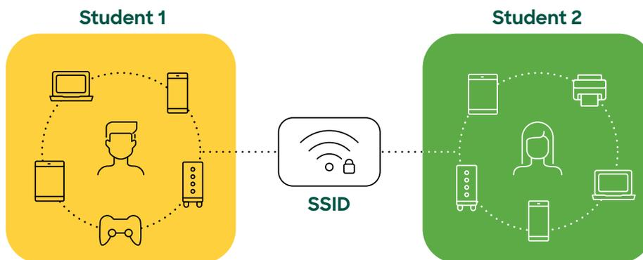
**WPN allows all user devices to authenticate to the SSID and communicate, creating a personal network**
